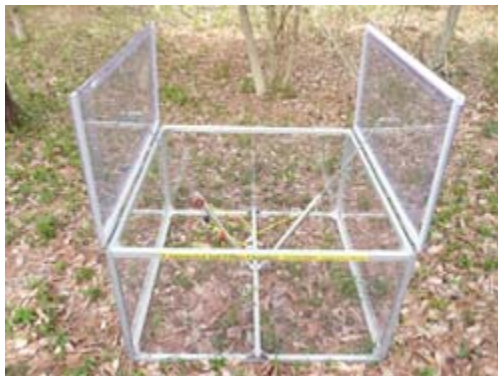
Fig.3. The standard automated chamber of LAC.
