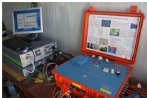
Fig.15. A multichannel LAC coupled with both CO 2 and isotopic CO 2 analyzers for measuring NEP and isotopic CO 2 flux at a Mongolian arid grassland site.
