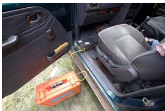
Fig.6. A micro powerful DC air compressor powered by a vehicle cigarette for filling the air tank inside the portable LAC.
