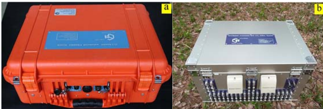
Fig.1. Control units of the multichannel automated chamber system. a: the unit for equipping maximum twelve chambers; b: the unit for equipping maximum twenty four chambers.
