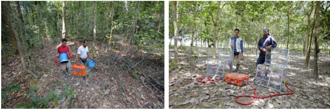
Fig.5. A portable LAC used in a Malaysian tropical forest (left) and a portable LAC equipped with two transparent automated chambers (right) used in a Malaysian rubber plantation.
